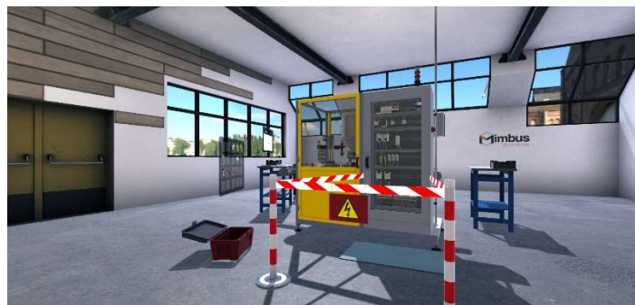
Figure 33 – Intervention area marked up
