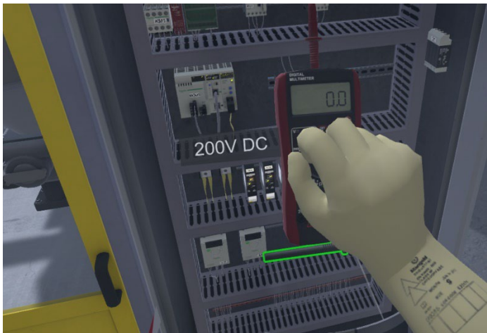
Measurements on the KM1 Contactor Between Terminals A1 and A2 (609-112)
