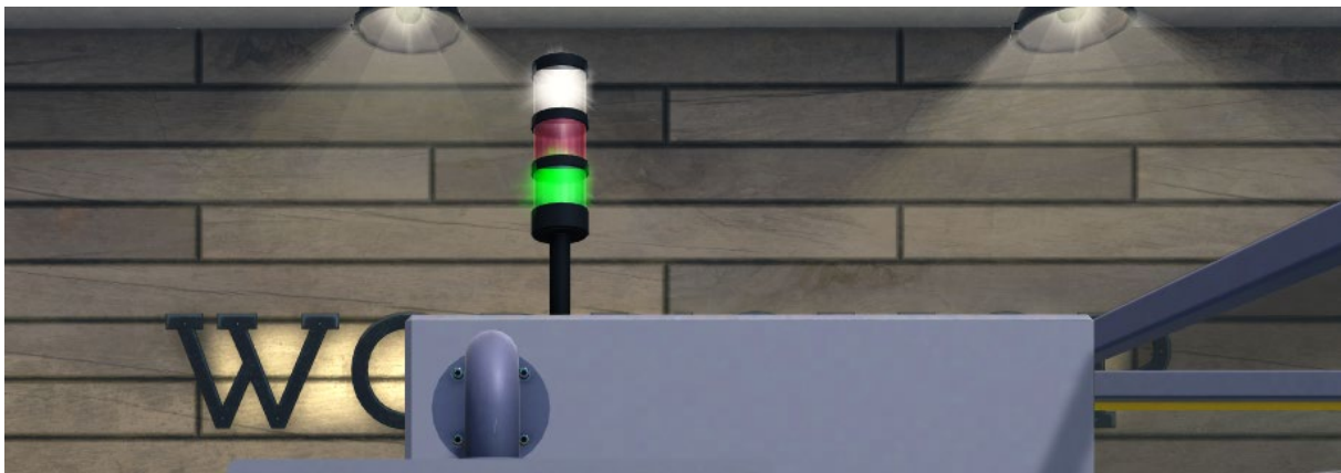
Figure 20 – Indicator lights when the machine works properly
